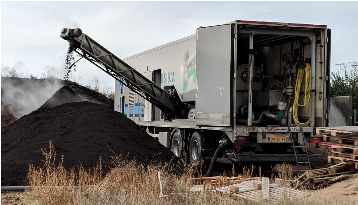
Figure 6. The EPM technology being used for on-farm swine manure dewatering.
