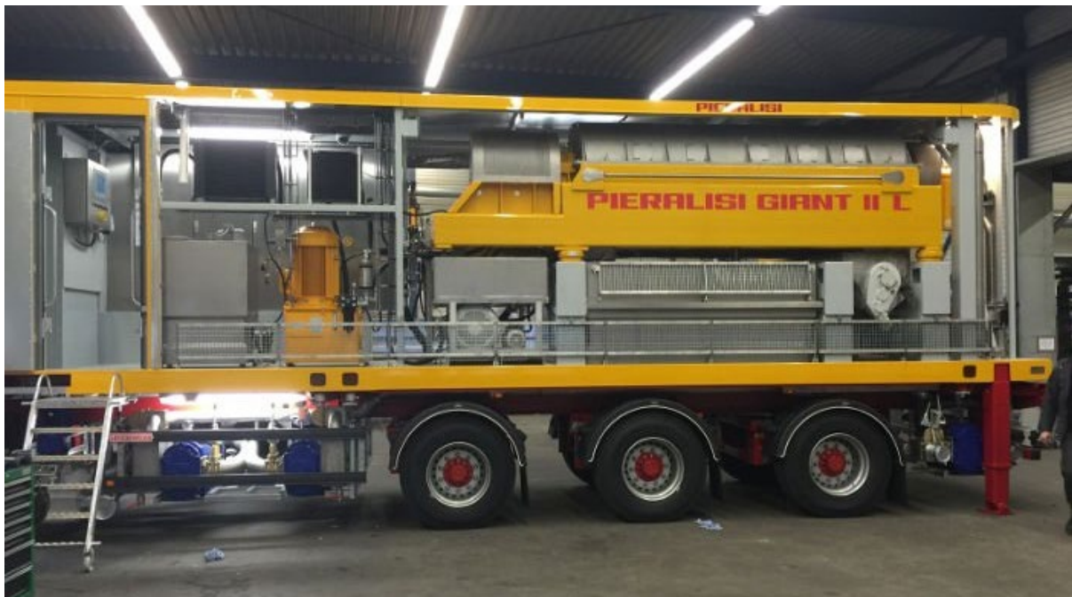
Figure 5. EPM Machining mobile slurry dewatering system under construction.
